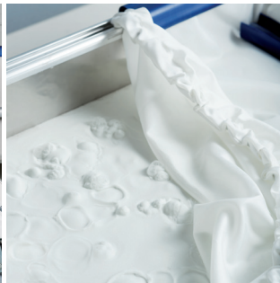
Fluidisation in progress
